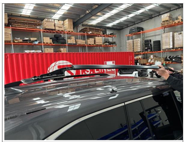
9. Remove the roof rail from the vehicle roof.
