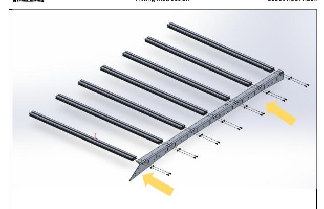
17. Fit the side rail to the extrusion,
